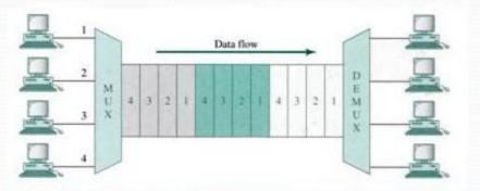
Portions of the signals 1,2, 3, 4 occupy the link sequentially.
