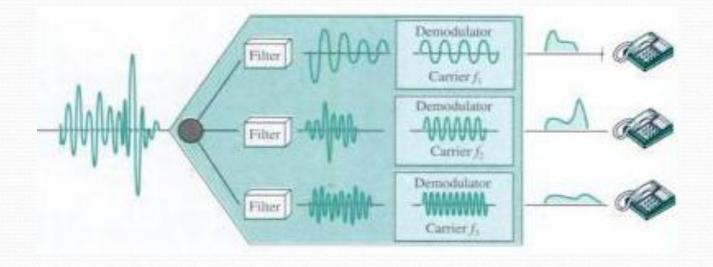
It uses a series of filters to decompose the multiplexed signal into its constituent component signals. Individual signals are then passed to a demodulator that separates from their carriers and passes them to the waiting receivers.
