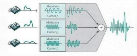
FDM is an analog process and we are showing here with the help of three telephones as input devices. Each telephone generates a signal of a similar frequency range. Inside the Mux, these similar frequency signals are modulated on different carrier frequencies, f1, f2, f3. the resulting modulated signals are then combined into a single composite signal that is sent out over a media link that has enough BW to accommodate it.
