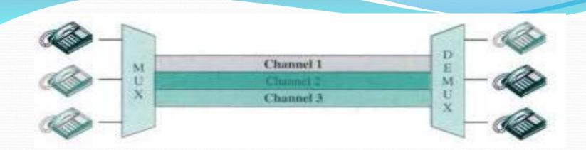
Transmission path is divided into three parts, each representing a channel to carry one transmission.
