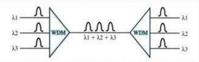
Very narrow bands of light from different sources are combined to make a wider band of light. At the receiver, the signals are seperated by the demultiplexer.
